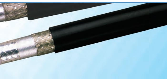
coverage single or double round wire braids. While these shields provide 40 dB and 60 dB shielding effectiveness respectively, they are not particularly stable (loss & vswr) nor is the shielding adequate for today's sensitive wireless communications and microwave military/defense applications.
