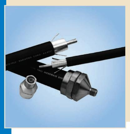
nu-TRAC TRC-1250 triaxial antenna cable is designed to provide controlled coverage in areas where RF propagation from a point source antenna is ineffective. Examples of common installations are subways, tunnels, ships, and metal framed buildings. The cable can function both as a transmit and receive antenna over a broad range of frequencies. The unique triaxial design allows for the cable to be mounted directly to a wall, thus eliminating cable standoffs and facilitating easy installation.
